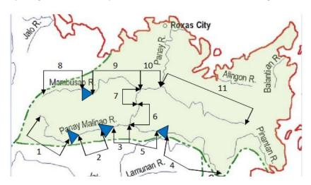
Figure 12: Eleven Reaches for Flow Model Inputs
